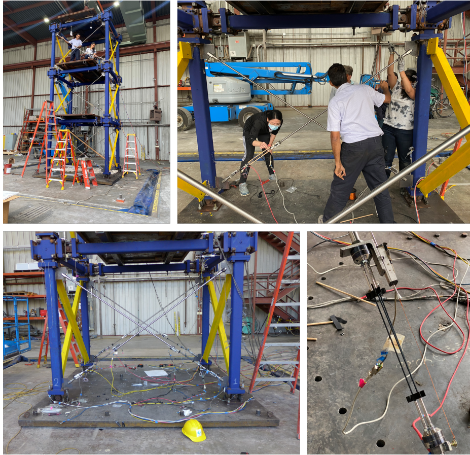
Fig. 2: Preparing instrumentation for the shaking table testing.
